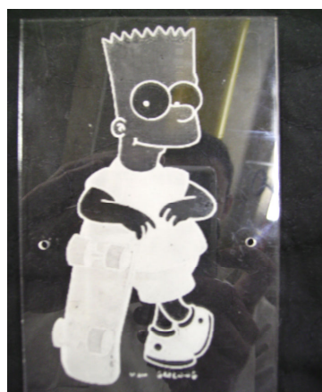
Figure 3 Laser engraved image onto clear acrylic
