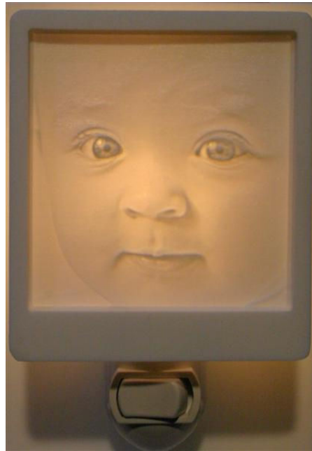
Figure 12 Lithopane machined from translucent plastic back-lit and mounted in a frame
