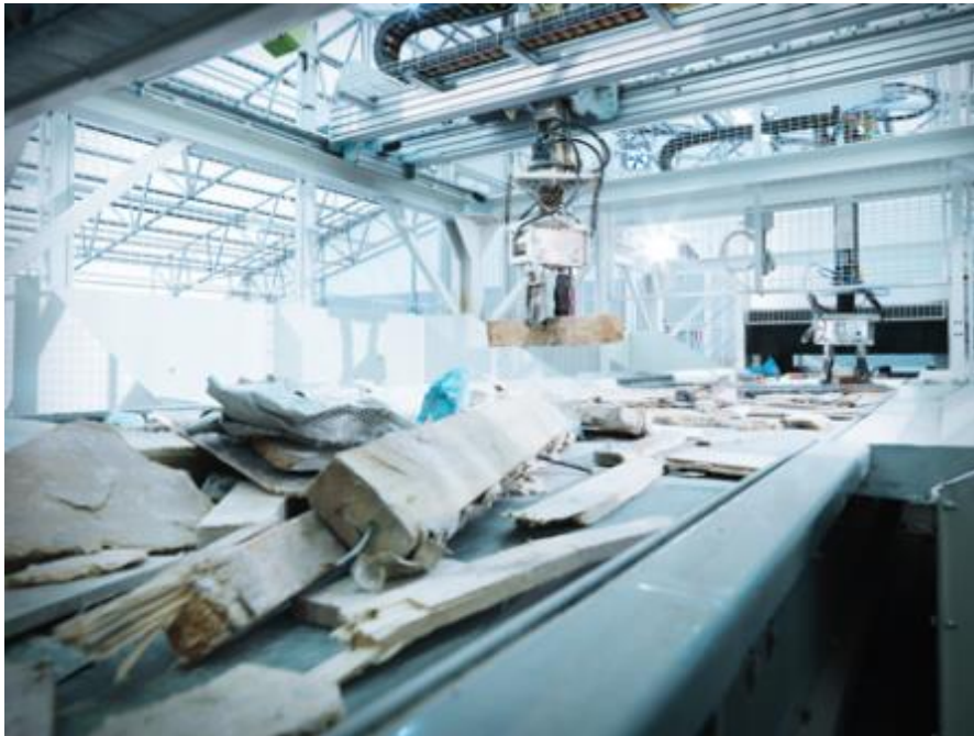
Figure 1: ZenRobotics Recycler sorting C&D waste
